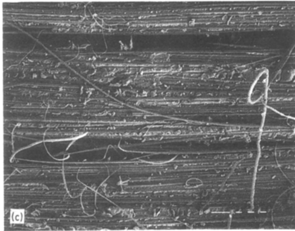
Figure 9 Scanning electron photomicrographs of the fracture surface in the aramid/epoxy layer of ARALL-1 laminates tested at the lowest strain rate ( 0.000\ 83\ \text{min}^{-1} ) and in the temperature range (a) 75\ ^\circ\text{F} ( 24\ ^\circ\text{C} ), (b) 180\ ^\circ\text{F} ( 82\ ^\circ\text{C} ), and (c) 250\ ^\circ\text{F} ( 121\ ^\circ\text{C} ) \times 100 .
